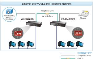
Refer to the following procedures to set up the VDSL2 Bridge LAN to LAN connection.
